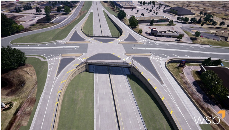
Caption: A key section of Minnesota's TH 169 in Elk River is being converted into a freeway, providing faster and safer access to Greater Minnesota. Image courtesy of WSB.
