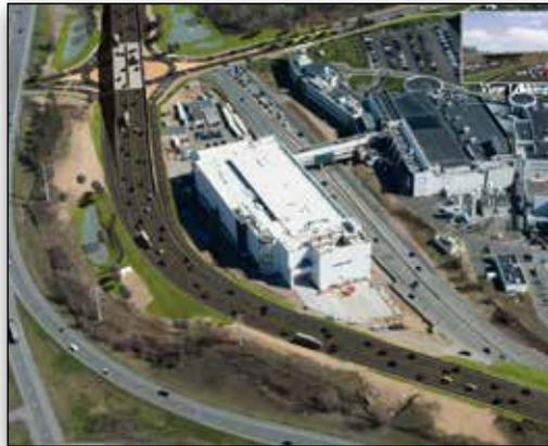
*Creighton Manning realigned Washington Avenue to incorporate two 95-foot-long, single-span bridges over a new two-lane roundabout on Fuller Road.*
