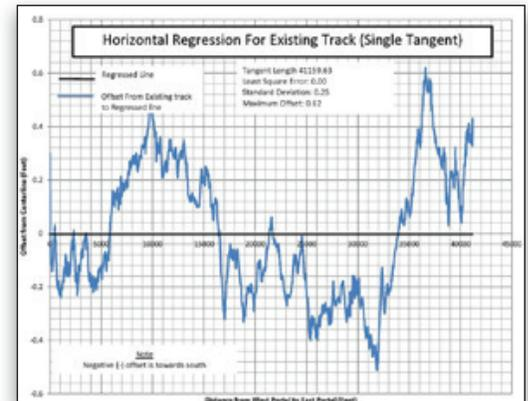
*Horizontal regression of existing track alignment with +ve and -ve offsets from centerline.*
