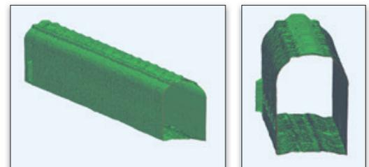
*3D PDF showing point cloud of tunnel surface with existing notches visible at top.*
