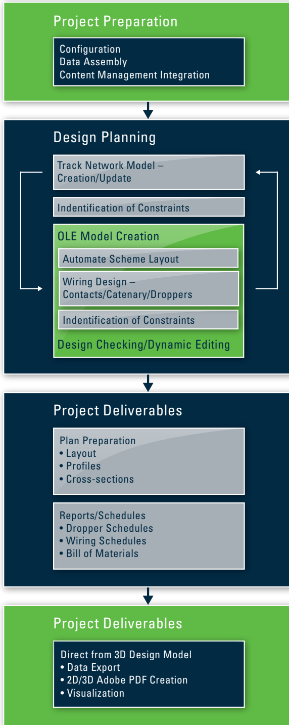
Overhead Line System – Design Process.
