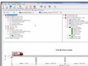
Drag and drop loads to define structure loads and load combinations for analysis.
