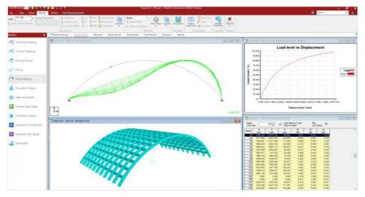
Geometric nonlinear analysis deformation.
