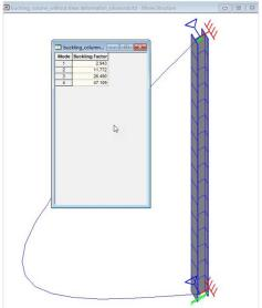
An eigen column buckling solution.
