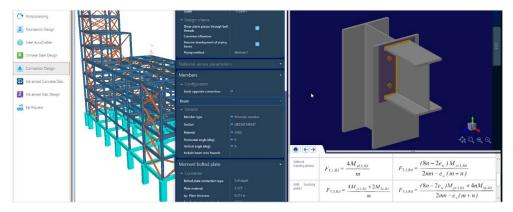
A typical beam-column flange connection.
