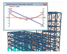
An example of a bending moment and shear force graph.
