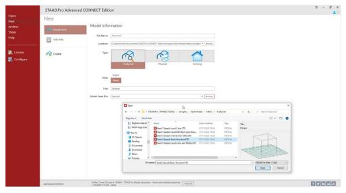
A new model setup with a sample model acting as the seed file.
