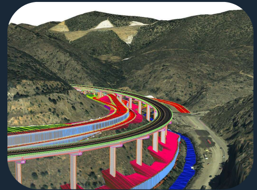
WB Viaduct and Reality Mesh
