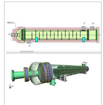
Designs for an AES type heat exchanger.
