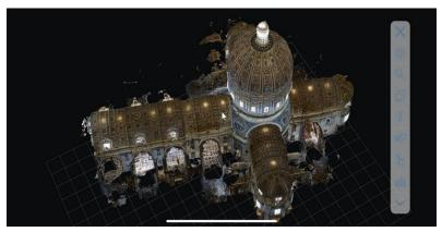
The project required an extensive survey campaign, resulting in a large amount of data needing to be managed and processed into a reality mesh, and shared among multiple disciplines and stakeholders for continued monitoring. To address these challenges on a six-month timeline, Italferr needed integrated and open 3D modeling and digital twin technology.
