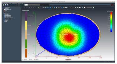
Simulated density changes in a geothermal reservoir, modeled and visualized in Flow State Solutions software Volsung. *Image courtesy of Flow State Solutions*.
