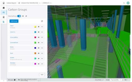
Design elements in logical groups for embodied carbon impact calculation. *Image courtesy of Bentley Systems*.
