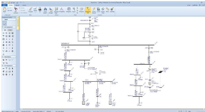
EasyPower’s intuitive interface empowers users to digitize their electrical systems, and enables design, analysis, and optimization of complex electrical power distribution systems. *Image courtesy of Bentley Systems.*
