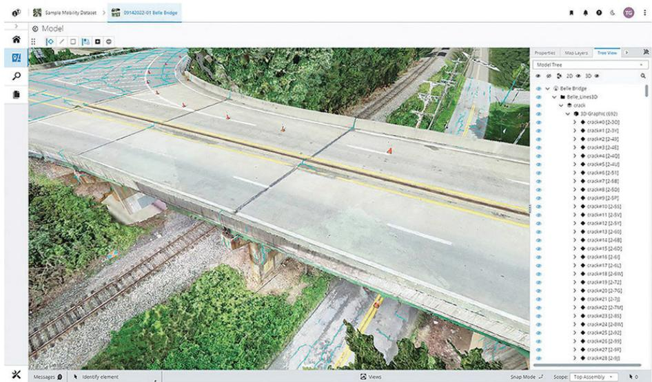
The iTwin Capture tool allows for digital twins to be built from drone imagery of assets.
