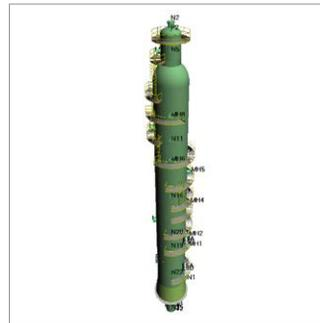
*Vertical pressure vessel with platforms
