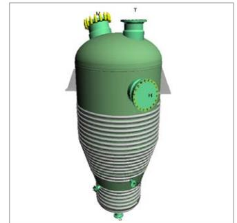
*Vessel with limpet coils.*
