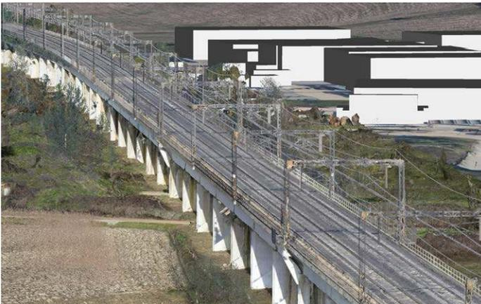
Italferr used ContextCapture to merge images on three flight planes to identify overlap and millions of tie points between them, resulting in a precise, high-resolution mesh.
