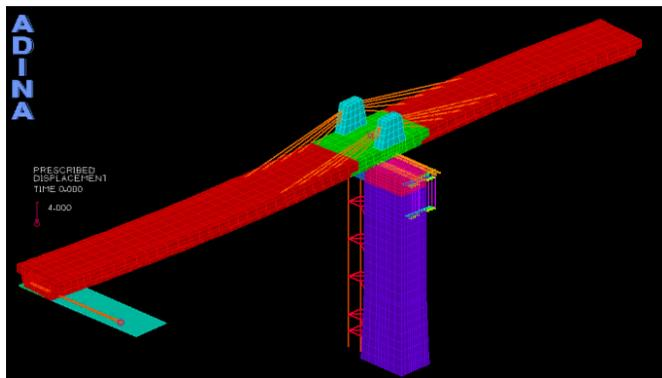
Caption: The frictional sliding of a prestressed concrete bridge girder can be studied with ADINA technology.
