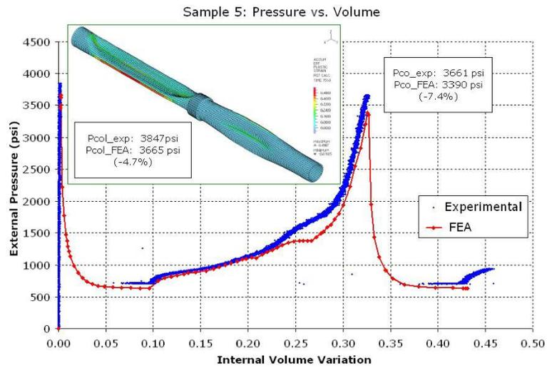
Caption: Collapse analysis of pressurized pipe can be performed with ADINA software.
