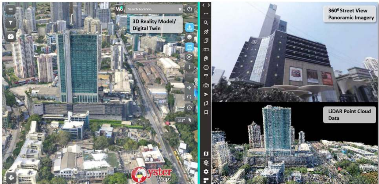
Oyster Maps, Genesys' In-house-developed 3D digital twin platform showcasing multiple datasets in parallel on a single window. Image courtesy of Genesys International.
