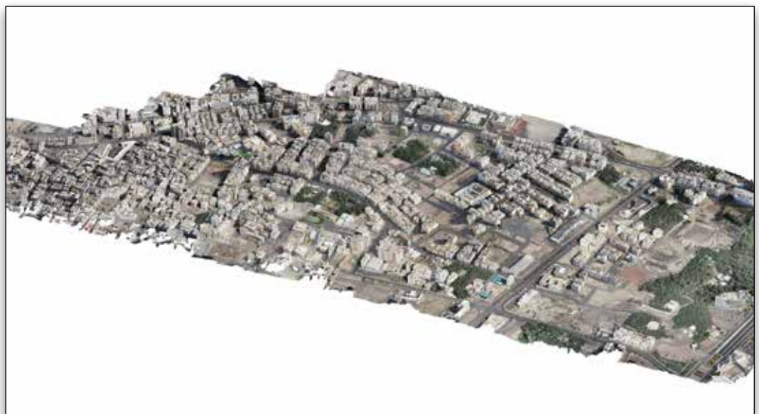
3D reality mesh of 216 sqkm of the Al Jumah District generated with ContextCapture.
