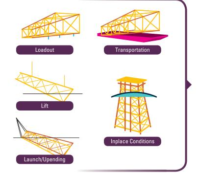
This new functionality allows the engineer to instantly view which design phase governs the design of each member and each joint.
