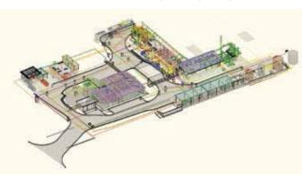
By using a shared data repository, **MWH** designers could do clash detections much earlier in the design process and save material costs. Santanu Das, Bentley SVP, Design **Modeling**
